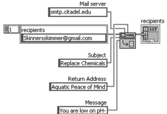
Fig. 7. LabView alert process
