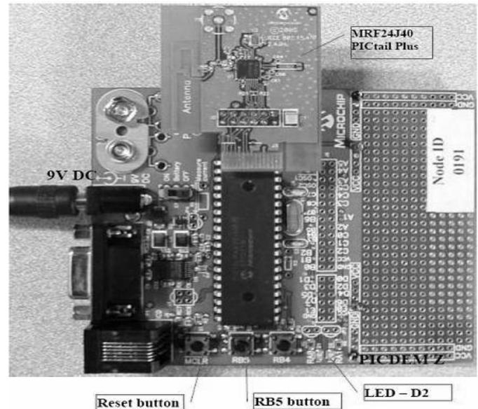
Fig. 4. PIC18F4620 project board with MRF24J40 PICtail Plus Zigbee module.
