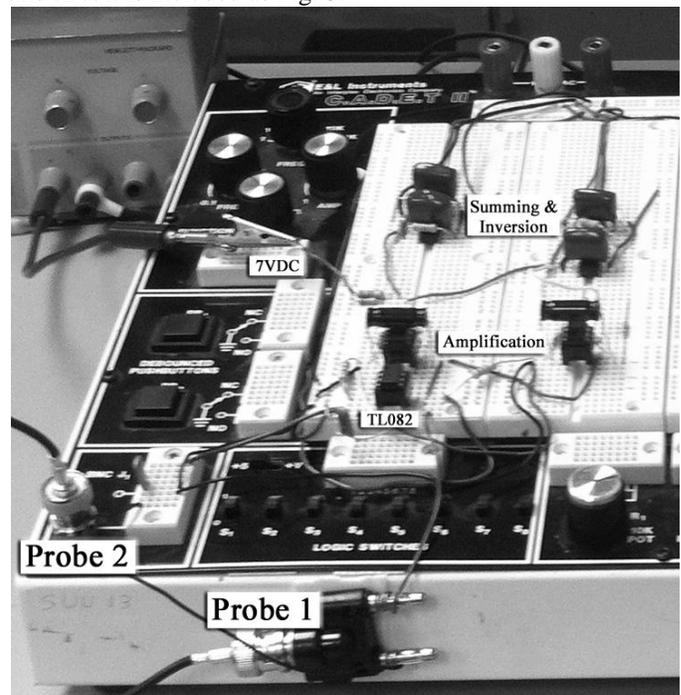
Fig. 3. Implementation of pH Metering circuit
