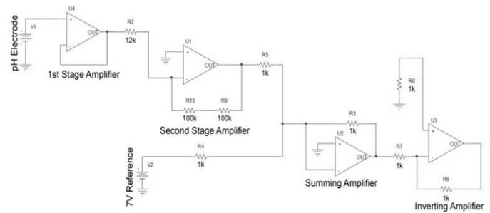
Fig. 2. Probe amplification schematic
