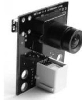
Fig. 5 - Vision Subsystem for NXT (NXT Cam) from Mindsensors.com, used for navigation.
