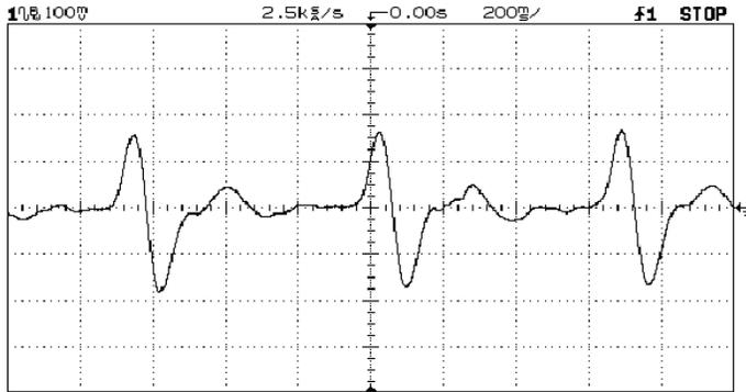
**Figure 2:** Wrist pulse sample (using Piezo Film Sensor)
