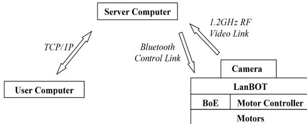
Fig. 1. LanBOT Functional system block diagram
