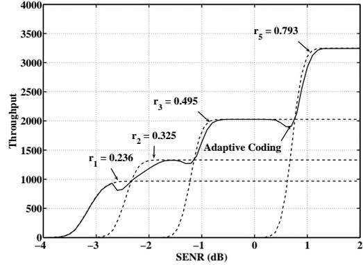
Figure 3. Performance of the adaptive protocol with the error count for 64-ary biorthogonal modulation
