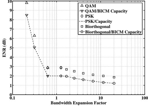
Figure 1. Relative performance of available modulation formats
