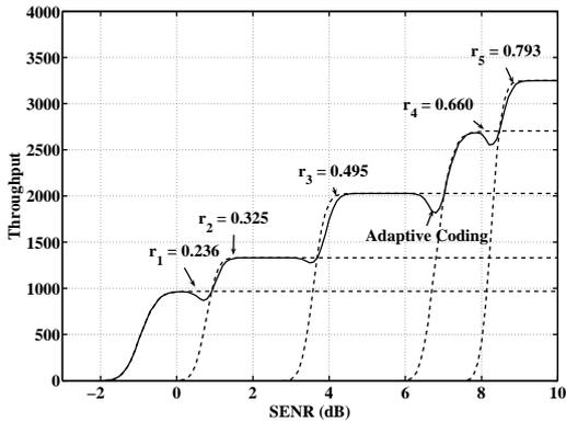
Figure 4. Performance of the adaptive protocol with the error count for 64-QAM
