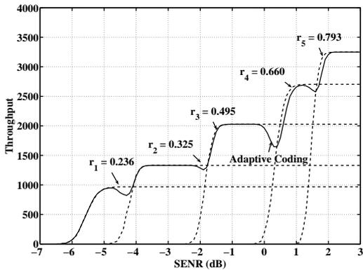
Figure 5. Performance of the adaptive protocol with the iteration count for BPSK
